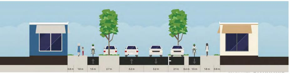
Figure 23. Internal loop road indicative cross section design (20m road corridor)
